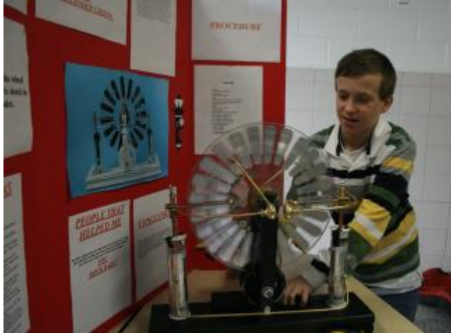
Alex showed off principles of static electricity using his homemade Wimshurst machine.
